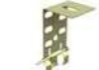
Direct suspension clip Chicago Metallic™ T-profile + securing pin H 100 mm max.weight 45 kg
